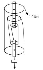
The diagram above shows a block and tackle pulley system of efficiency 80%. It is used to raise a load through a height of 20m with an effort of 100N. Find the energy wasted.
